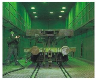
abrasive being shot at the work piece, as well as providing lighting and ventilation for the operator's safety.
